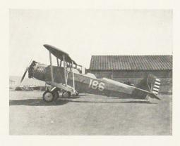
Very new and modern Douglas 0-32A, powered with Wasp motor, used for advance Army training and observation
